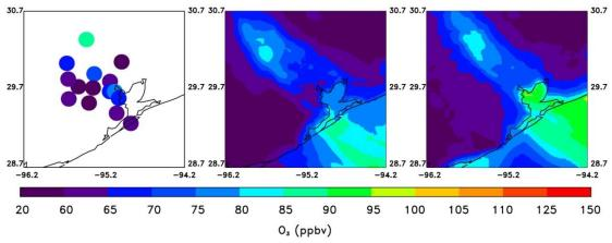
Figure 3: Eight hour average ozone maximum from observations (left), original 4 km CMAQ simulation (middle), and new 4 km CMAQ simulation on 26 September 2013.
