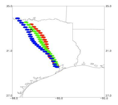
Figure 5: Back trajectories from the new 4 km WRF model output initialized at La Porte Sylvan Beach at 20 UTC at 0.5 km (red), 1 km (green), and 2 km (blue) AGL. The letter 'D' shows the location of Dallas, TX.
